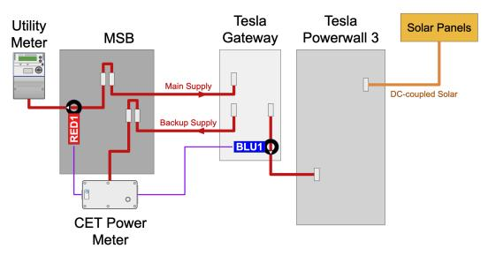
The CET Power Meter should be powered from the backup supply.
