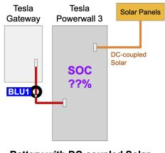
Battery with DC-coupled Solar HEMS can not see power going to battery from panels, unknown SOC %
